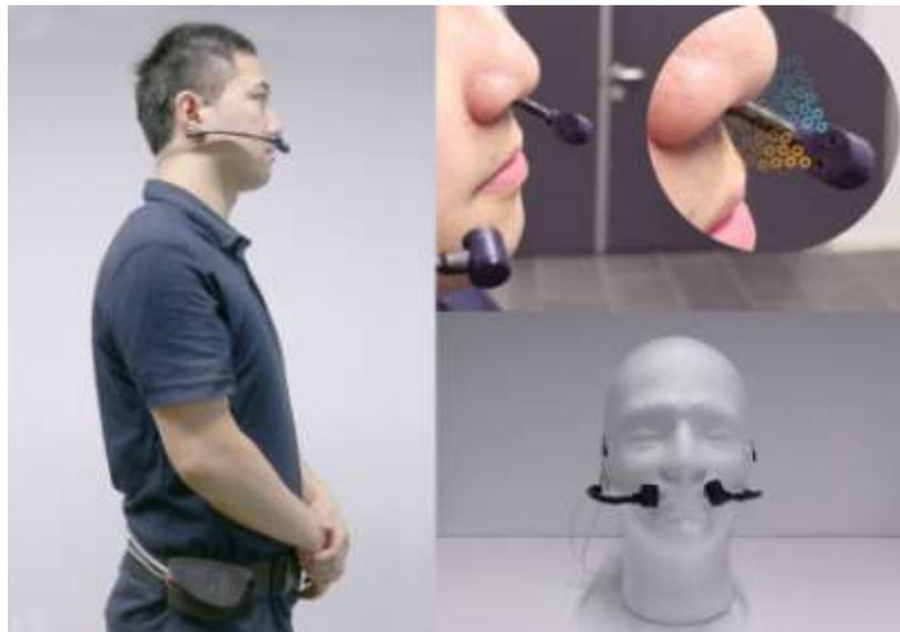
**Description:** This device is a wearable Olfactory Display, tiny and comfortable to wear, which can deliver 4 different odors, and can be connected to a wireless app for mobile applications.
