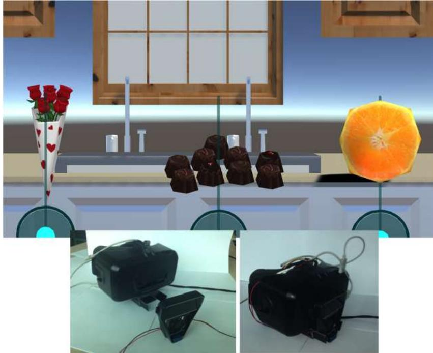
**Description:** The application allows the user to see objects through a stereoscopic head mounted display, to interact with virtual objects through hand gestures detected by a LeapMotion sensor and to smell odors associated with the objects when grabbed delivered by an Olfactory Display integrated with the display.
