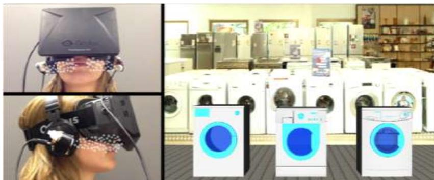
Description: The application allows designers to evaluate in which way odors can influence the users' evaluation of products. The application shows some washing machines in a store, and users should tell preferences. The evaluation is performed with and without odours.
